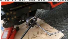
H. Get your socket & add Loctite to the stude on the spacer. Install the rim/wheel & now use the new nuts from the spacer, making sure they are flip to the proper end. Torque the nuts to 90 ft. lbs for the rim in the same 3 steps as above (3/4" Socket).
