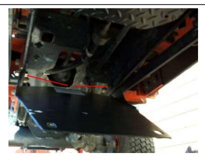
.7 Check everything out for clearances & binding. Recheck nuts & bolts every month. If attachment is installed, check their clearances with the skid plates (put the 3pt in the lowest & highest position.
