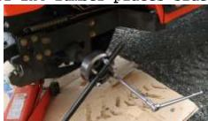
careful not to damage the wheel spacers stud /treads
