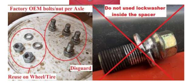
do not mix these up. You should now have 2 factory nuts/lock washer. Disregard the 4 factory bolts/lock washer. We supplied new Lock Washer for the install of the wheel. In Step "H" to install the rim Do not use the OEM factory bolts or nuts to install the spacer to the axle. We supplied 4 New Gold taper lug Bolts per side & take from the spacer 2 of the 6 new gold Nuts from the spacer.
