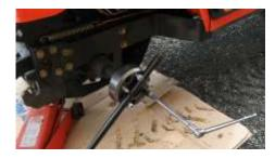
The factory bolts threads are 14mmx2 thread, we have supplied new Lug bolt 14mmx2 use these to install the spacer to the axle
