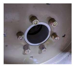
H. Check clearances around the Wheel, no point of contact should be noticed.
