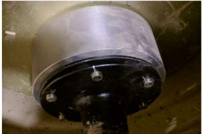
Using the "Paint pen" leave a line going from the backside of the axle flange onto the end of the treads lug bolts. Do the same on the outside of the wheel side. This way if the lug bolts break themselves lose, the paint line will no longer align, warning you of needing retorque everything up.
