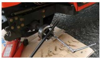
H. Get your socket & add Loctite to the studs on the spacer. Install the rim/wheel & now use the new nuts from the spacer, making sure they are flip to the proper end. Torque the nuts to 90 ft. lbs for the rim in the same 3 steps as above (3/4" Socket).
