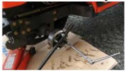
H. Reinstall the wheel & torque the nuts to 70 ft. lbs for the rear wheels.
