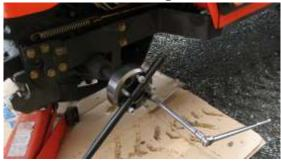
H. Reinstall the wheel & install use the new nut we supplied & Torque the new nuts to 60 ft. lbs for the front wheels.
