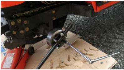
H. Get your socket & add Loctite to the studs on the spacer. Install the rim/wheel & now use the new nuts from the spacer, making sure they are flip to the proper end. Torque the nuts to 110 ft. lbs for the rim in the same 3 steps as above.
