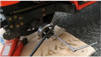
H. Get your socket & add Loctite to the studs on the spacer. Install the rim/wheel & now reuse your factory OEM nuts Torque the nuts to 110 ft. lbs for the rim in the same 3 steps as above.
