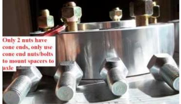
Please take the time to make the install in 3 steps. First hand tightens the bolts; Second torque the bolts to half the torque in a crisscross pattern & finally torque the bolt to their final value of 150 ft. lbs for the rear's wheels.
