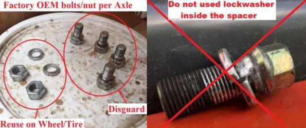
🛆 do not mix these up. You should now have 2 factory nuts/lock washer. Disregard the 4 factory bolts/lock washer. We supplied new Lock Washer for the install of the wheel. In Step "H" to install the rim  $\triangle$  Do not use the OEM factory bolts or nuts to install the spacer to the axle. We supplied 4 New Gold taper lug Bolts per side & take from the spacer 2 of the 6 new gold Nuts from the spacer.
