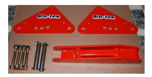
For the first time around, install the top two bolts (some thumbs only require 1), Lock nut & Washer. Do not tight it all the way, like the one in photo.
