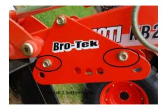
E. Push the two plates away from the bucket, until the bolts snug up against the boom. Tighten the 3 or 4 bolts snug.
