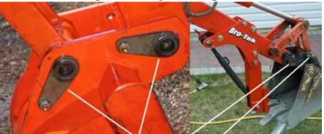
BX24 has a new setup for the pins, the BX22 & BX23 pins have one hole drill at one end, which a bolt holds the pin in place.
