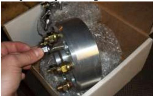
Now is a good time to test fit the spacer to the Axle & then to the wheel rim. The spacer should make full contact to the axle, it's much easier to sort any problems without having anything bolted down.
