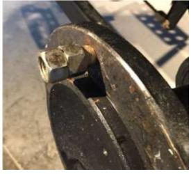
You will need to remove the 2 Stud on the axle, double nut tight the Stud as in photo & turn counter clockwise the inside nut. The stud should unscrew itself from the axle.
