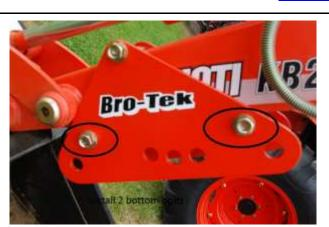
E. Push the two plates away from the bucket, until the bolts snug up against the boom. Tighten the 3 or 4 bolts snug.
