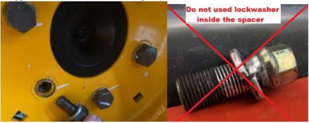
⚠ Disregard the 6 factory bolts/lock washer. We supplied new Lock Washer & lug bolt for the install of the wheel. In Step "H" to install the rim
